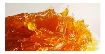
The primary function of grease is to coat the machine surfaces and to lubricate them without leakage due to centrifugal forces or pressures. Also, grease must be able to flow throughout all components it is intended to.
