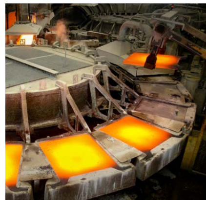
Liquid copper solidifies in the square moulds of the casting wheel.
