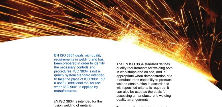
EN ISO 3834 is intended for the fusion welding of metallic materials, and its application is independent of the products manufactured. However, its principles and many of its detailed requirements are also relevant for other welding and welding-related processes.
