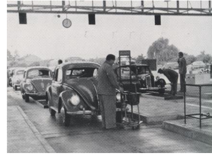
Lights test of a car with Bosch test device
