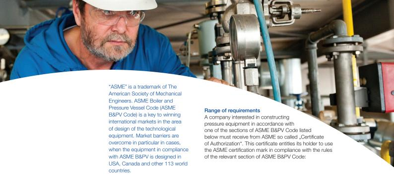
ASME ASME B&PV Code sets requirements for the certification of producers of equipment, a control system / quality assurance, design, production, testing and certification of boilers and their pipeline systems, pressure vessels and nuclear facility components.
